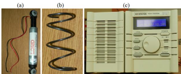
Fig.3. MR damper RD 1097-01 (a), SMA nitinol spring (b) and power supply PSH 3620A dedicated for SMA spring (c)
