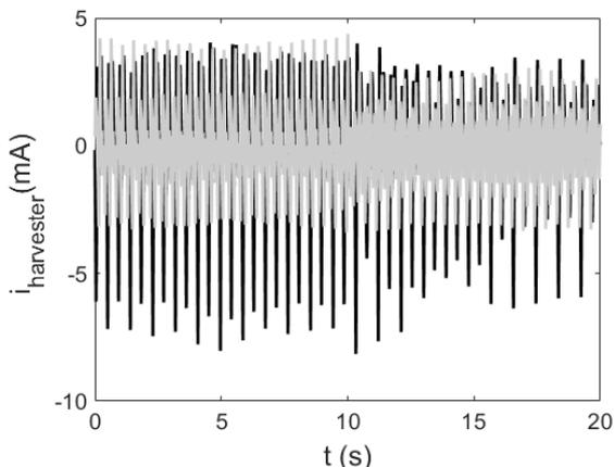
Fig.6. Time series of current  $i_{harvester}(t)$ . Black line - pendulum is activated, gray line - pendulum is non activated. Switch MR damper control from *off* to *on* at  $t=10$ s. Parameter  $\gamma=0.09$
