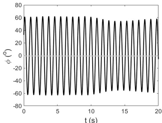
Fig.4. Time series of angle  $\phi(t)$ . Black line - pendulum is activated, gray line - pendulum is non activated. Switch MR damper control from *off* to *on* at  $t=10$ s. Parameter  $\gamma=0.09$ .
