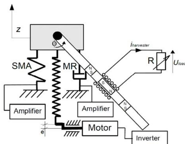
Fig.2. A scheme of the experimental setup
