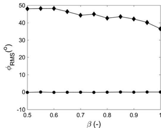
Fig.9. The RMS value of pendulum rotate via parameter  $\beta$ . Circle marker – pendulum non activated, diamond marker – pendulum activated
