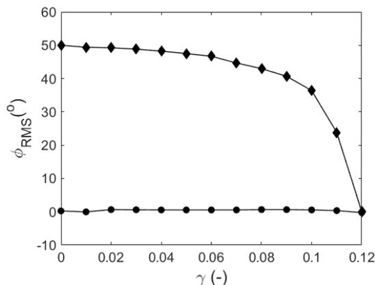
Fig.7. The RMS value of pendulum rotate via parameter  $\gamma$ . Circle marker – pendulum non activated, diamond marker – pendulum activated
