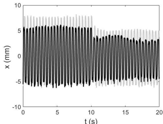
Fig.5. Time series of displacement  $x(t)$ . Black line - pendulum is activated, gray line - pendulum is non activated. Switch MR damper control from *off* to *on* at  $t=10$ s. Parameter  $\gamma=0.09$ .
