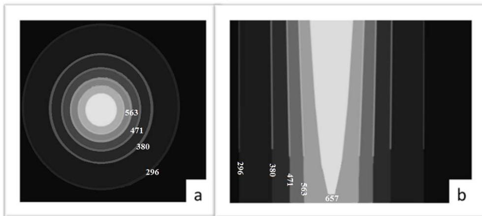
Fig.1. Contour maps of temperature field on the border of the Ni-based coating and the Fe-based substrate: the section cut parallel to the plane of the sample surface (a); the section cut perpendicular to the plane of the sample surface, the vector of the beam velocity is parallel to the plane of the cut (b)
