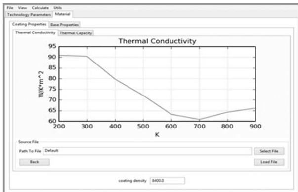
Fig.2. The screenshot of the window of thermophysical properties of the coating material: the graph of Nickel thermal conductivity coefficient dependence on temperature
