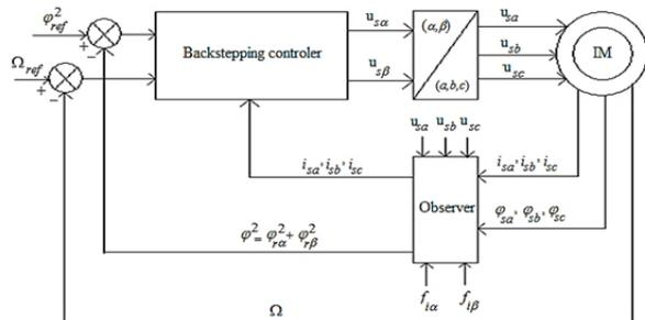
Fig.3. Scheme of the backstepping with an observer.
