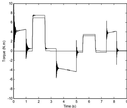
Fig. 6. Motor and load torque with observer,  $\theta = 10$ .
