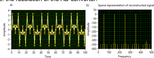
Fig. 3. The segments of time waveforms of the original (white line) and reconstructed signal (dotted yellow line) (a) and normalized DFT components of the reconstructed signal (b). The set no 1
