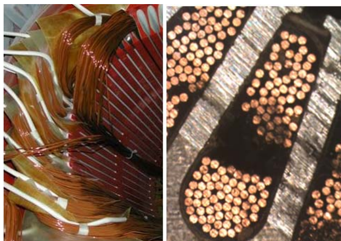
Fig. 6. Deep slots for auto-wound double-layer windings with parallel paths are not recommended. Winding asymmetries due to coil side locations in the slot lead to unequal impedances and unequal induced EMFs.
