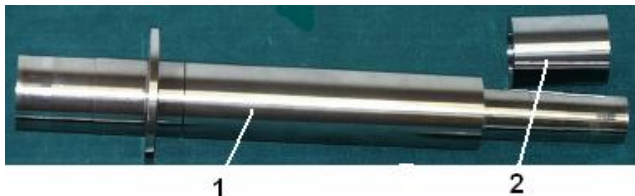
Fig. 9. Rotor of a 100 kW, 70 krpm PM brushless motor for an oil free compressor. 1 – PM rotor with retaining sleeve, 2 – foil bearing journal sleeve. Photo courtesy of Mohawk Innovative Technology, Albany, NY, USA.
