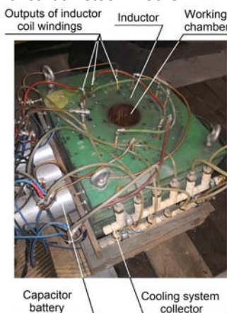
Fig.4. Electromagnetic mill inductor prototype (photo provided by MEGATECH Zbigniew Gałuszkiewicz)
