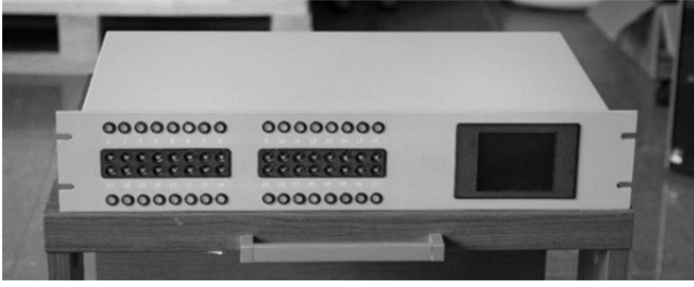
Fig.2. An electrical tomograph for measurements in electrical tomography.
