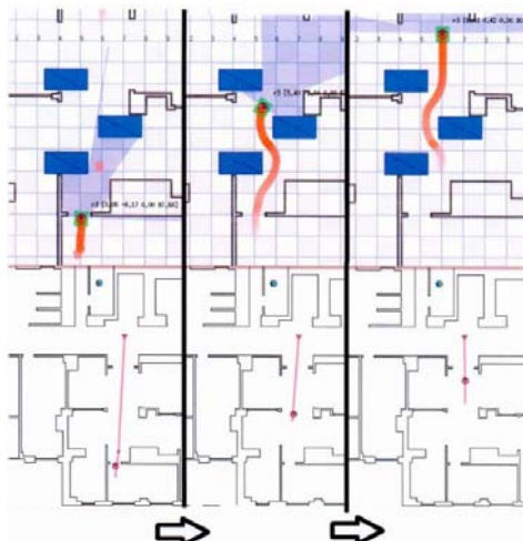
Fig. 8 Simulated robot dynamic obstacle avoidance
