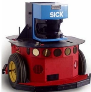
Fig. 7 Pioneer 2DX with Sick LMS200 laser scanner
