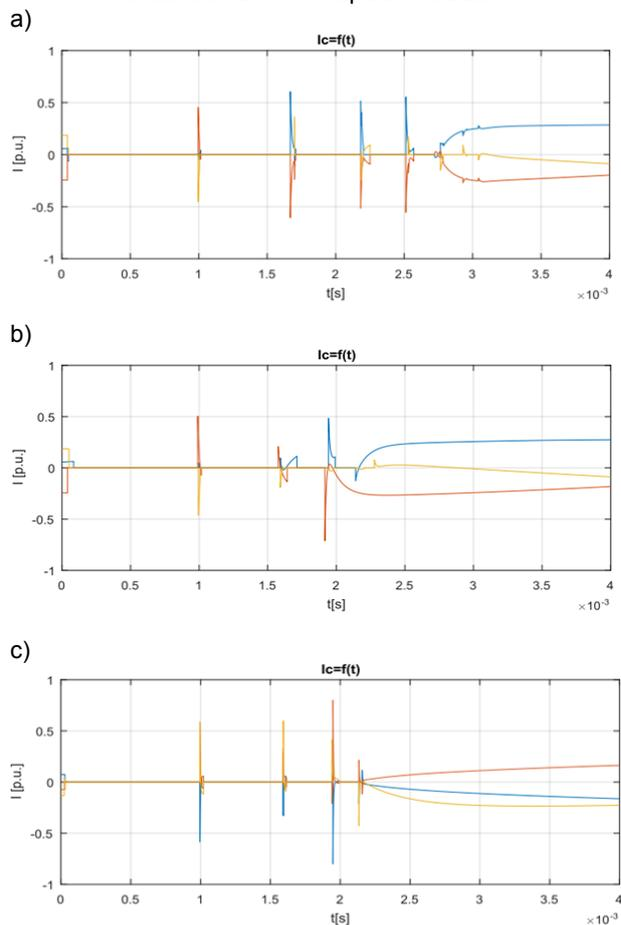
Fig. 10. Waveforms of  $I_c$  current that flows through a capacitor bank. Circuit parameters: bank power  $Q = 50 \text{ MVar}$ , supply voltage  $U_z = 8 \text{ kV}$ . Capacitor bank connection systems: a) star b) star with a grounded neutral point c) delta
