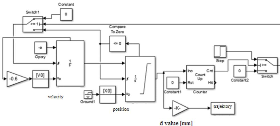
Fig.5 Algorithm simulating the elastic bounces of a contact
