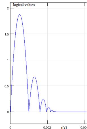
Fig.4 Simulation of the bounces of a movable contact in a vacuum circuit breaker
