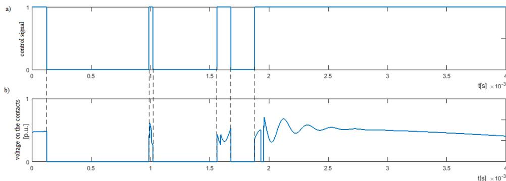
Fig. 8. Influence of the control signal (a) on the voltage at the capacitor clamps (b)
