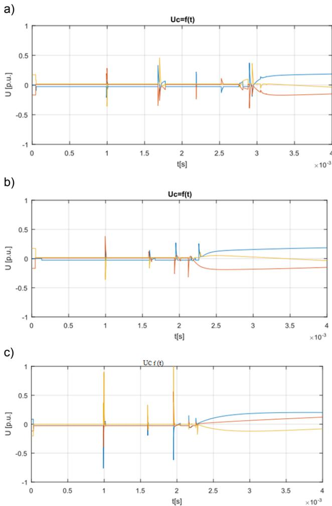
Fig. 11. Waveforms of  $U_c$  voltages on the capacitor clamps. Circuit parameters: bank power  $Q = 50 \text{ MVAR}$ , supply voltage  $U_z = 6 \text{ kV}$ . Capacitor bank connection systems: a) star b) star with a grounded neutral point c) delta
