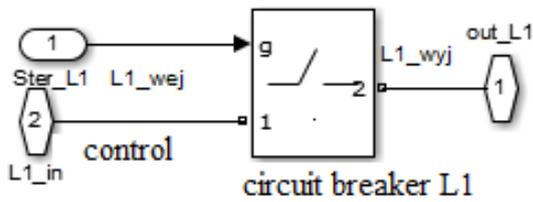
Fig.1 Scheme of one of the poles of a circuit breaker
