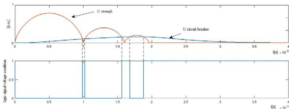
Fig. 7 Scheme of operation of the voltage element of the algorithm that generates the signal that controls the poles of the circuit breaker
