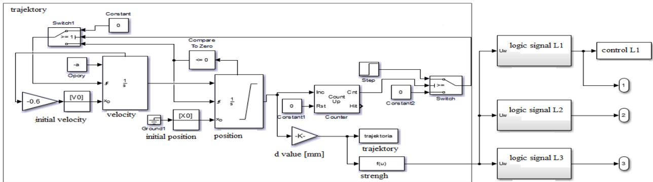
Fig.2 Control system of the trajectory poles of a circuit breaker
