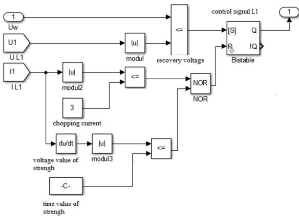
Fig.3 Voltage and current conditions for controlling the pole of a circuit breaker
