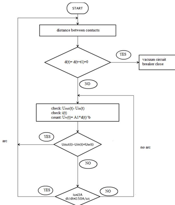
Fig.6. Algorithm of the system controlling the poles of a circuit breaker
