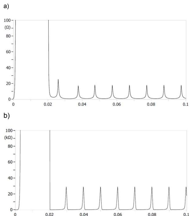
Fig. 9. Arc resistances; a) a grid with a directly grounded neutral point; b) grid with isolated neutral point.
