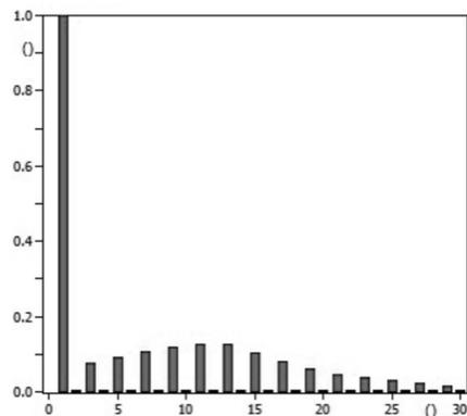
Fig. 6. Spectrum of higher harmonics of current for arc fault in a grid with isolated neutral point
