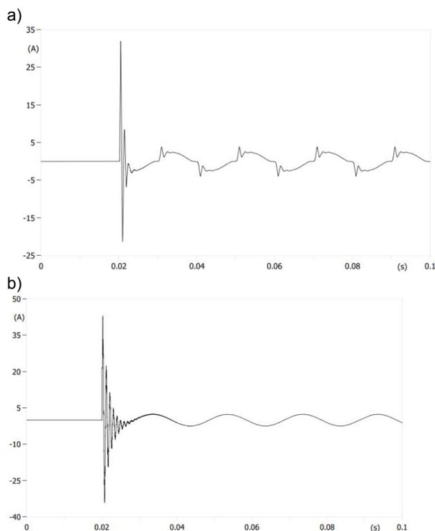
Fig. 5. Arc current in the grid with insulated neutral point; a) arc fault; b) short circuit via the transition resistance  $R_f = 0.01 \Omega$
