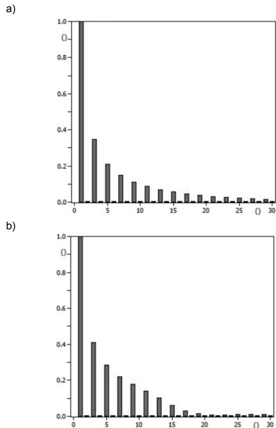
Fig. 8. Spectrum of higher voltage harmonics; a) a grid with a directly grounded neutral point; b) grid with isolated neutral point.
