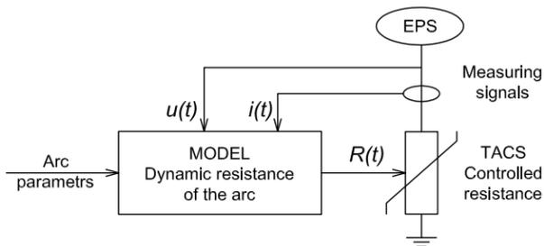
Fig. 1. Block diagram presenting the arc model in the EMTP-ATP program
