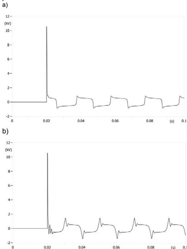
Fig. 7. Arc voltage: a) a grid with a directly grounded neutral point; b) grid with isolated neutral point
