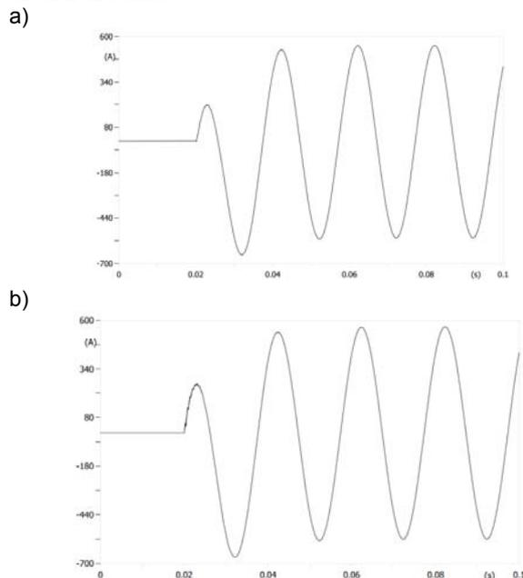
Fig. 4. Arc current in the grid with a directly earthed neutral point; a) arc fault; b) short-circuit via the transition resistance  $R_f = 0.01 \Omega$
