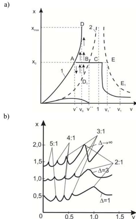
Fig. 10. Amplitude-frequency characteristics of the system in the superharmonic vibration mode:
