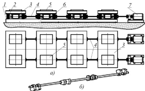
Fig. 12. Vibration machine for generating multiphase vibrations
