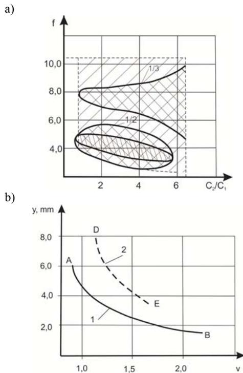
Fig. 9. Subharmonic vibrations in the vibration machine-medium system: a) area of subharmonic vibrations in coordinates  $f$  and  $c_2/c_1$ ; b) Amplitude-frequency characteristics  $y = f(v)$ ; 1 - for the basic vibration frequency; 2 - for the frequency with a freq. ratio of 1:2
