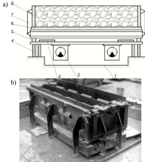
Fig. 3. Resonance shock-and-vibration machine for forming concrete foundation blocks: a) – Schematic diagram; b) – Construction design; 1 – Lower frame; 2 – Vibration exciter; 3 – Vibration limiter; 4 – Vibration-isolating support; 5 – Spring support; 6 – Pan; 7 – Equipment for closing and opening the side plates; 8 – Side plate
