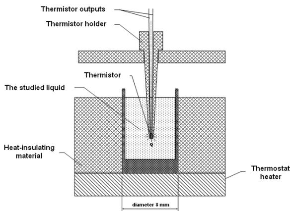
Fig. 1. Location of the thermistor probe and the test in studies of TPC fluids
