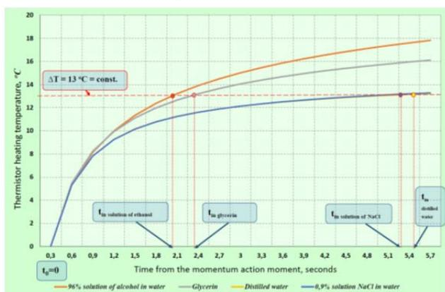
Fig. 7. Method of determining the time of additional thermistor heating to a temperature of 13°C in different investigated fluids.
