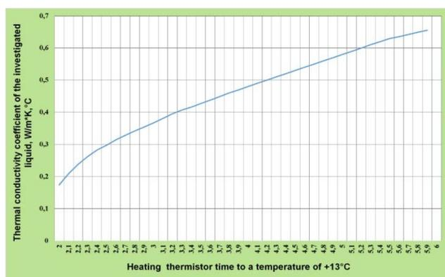
Fig. 8. Measured in the testing process, the real dependence of the value of the thermal conductivity coefficient for studied fluids from the time of thermistor heating to a temperature of 13°C.
