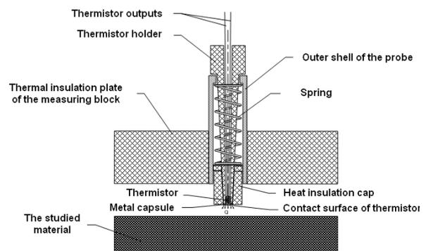
Fig. 2. Location of the thermistor probe and the test substance in studies of solid phase TPC
