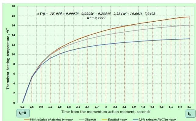
Fig. 4. Thermistor heating thermograms in  $T=f(t)$  of various substances (96% solution of ethyl alcohol, glycerol, distilled water, 0.9% NaCl solution in water).
