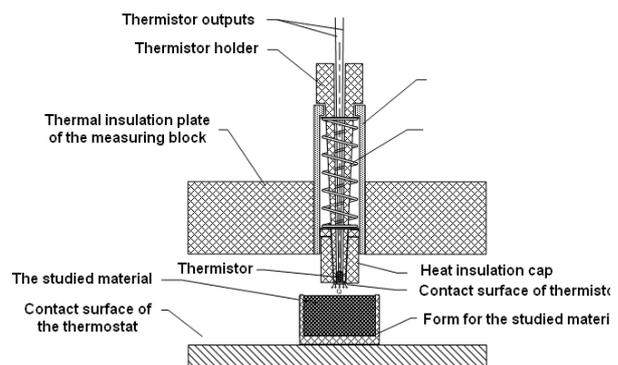
Fig. 3. Location of the thermistor probe and the test substance in TPC studies of conditionally solid and bulk materials [13]
