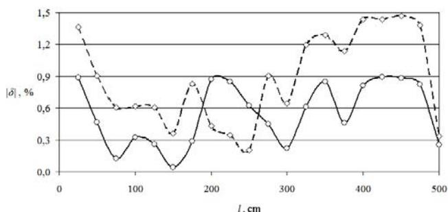
Fig.4. Dependence of absolute values of the relative error  $|\delta|$  from the measured distance  $l$ : with consideration of environmental parameters —○ and without consideration of environmental parameters ---◇
