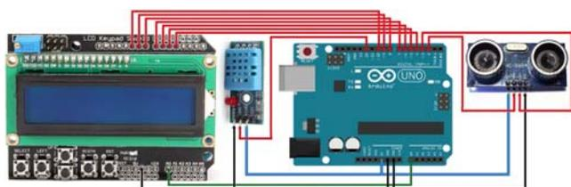
Fig.3. Connection of the indicating and controlling module, the sensor for distance measuring with consideration of environmental parameters to the Arduino Uno R3 board
