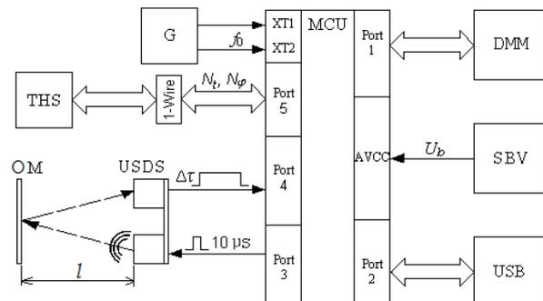
Fig.1. The structural diagram of the device for distance measuring with consideration of environmental parameters
