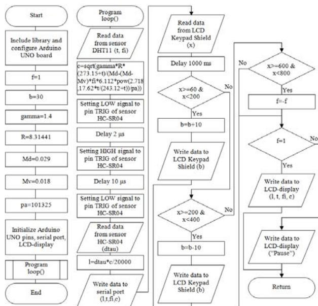
Fig.2. Block scheme of the main program algorithm and the loop program
