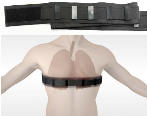
Fig.2 A photo of a measuring strip with installed measuring electrodes and a visualization of its location on the chest.
