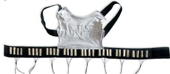
Fig.3. Measuring system based on textile electrodes with signal cables.
