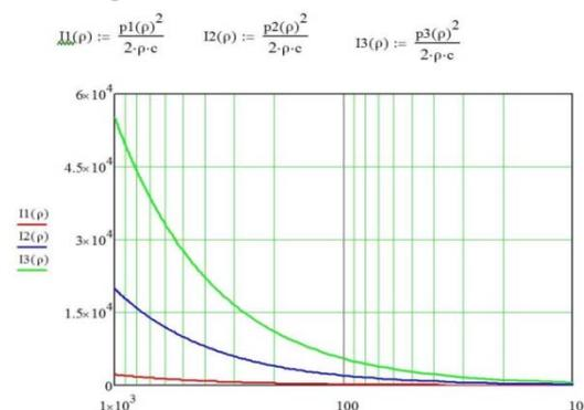
Fig.1. The dependence of the intensity of the sound  $I$  on the density  $\rho$  for the three values of the amplitude of oscillation  $A$
