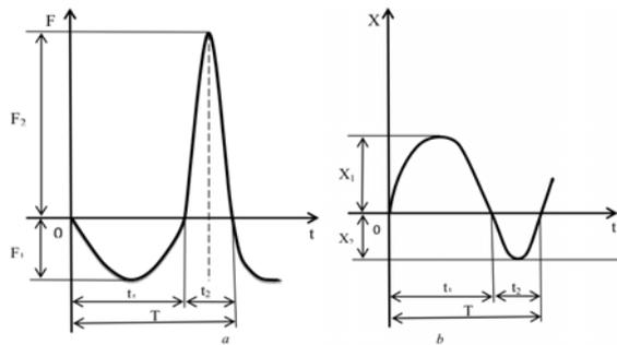
Fig.5. The nature of the change in the force F (a) and the displacement of X (b) in the contact zone under pulsed loading conditions
