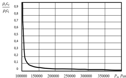
Fig.3. Dependence of the relative wave resistance of the environment on the sound pressure
