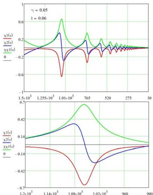
Fig.4. Change of contact pressure  $\chi \chi^{1(c)}$ , wave coefficients  $\chi^{1(c)}$  and  $\chi^{2(c)}$  depending on the waves velocity  $c$  in water with its ultrasonic cavitation treatment: frequency 24 kHz, coefficient of energy dissipation in the environment  $Y = 0.05$ , acoustically limited environment  $l = 0.06$  m; a – on the entire processing stage; b – within the limits of the first resonance
