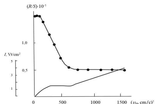
Fig.2. The dependence of the effective water resistance (curve 1) and the actual intensity of the sound (curve 2) on the square of the vibrational velocity of the cavitation apparatus
