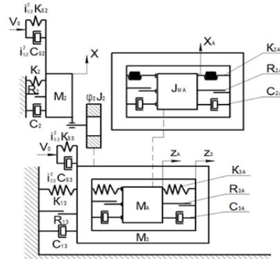
Fig. 4 Dynamic model of operative cycle
