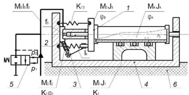
Fig. 1. Structural scheme of hydropulse vibromachine
