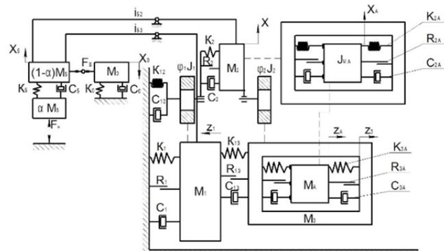
Fig. 2 Complete dynamic model of vibration machine
