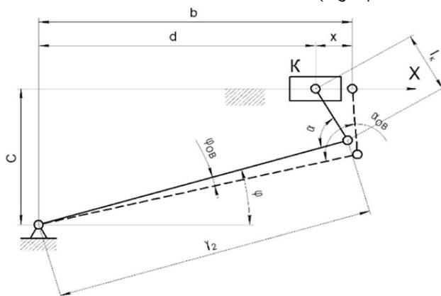
Fig. 5. Calculation diagram of the slide-crank mechanism of steering device
