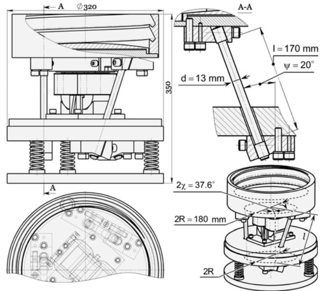
Fig. 6. General view of the vibration bunker Feeder
