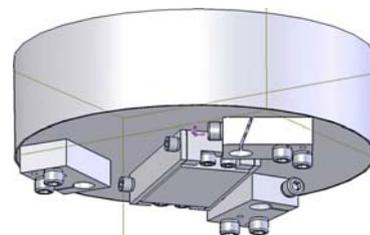
Fig. 7. Bowl, the mass of which is  $m_1 = 22.8 \text{ kg}$ , and the moment of inertia relative to the axis of rotation  $J_1 = 0.29 \text{ kg} \cdot \text{m}^2$
