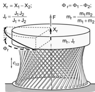
Fig. 5. An oscillation system based on a hyperboloid torsion, reduced to single weight
