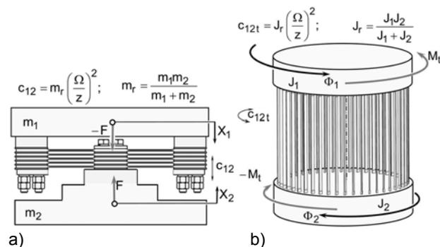
Fig. 3. Oscillation systems with rectilinear (a) and angular (b) movement
