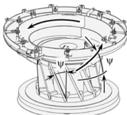
Fig. 1. Vibrating bunker feeders with guided (screw-like) oscillations in which the bowl is made cylinder-like (a) and a conical-like (b)
