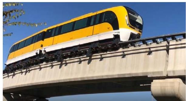
Fig. 2. The maglev trainset on elevated guideway. Photo taken near maintenance depot (Yongyu Station).
