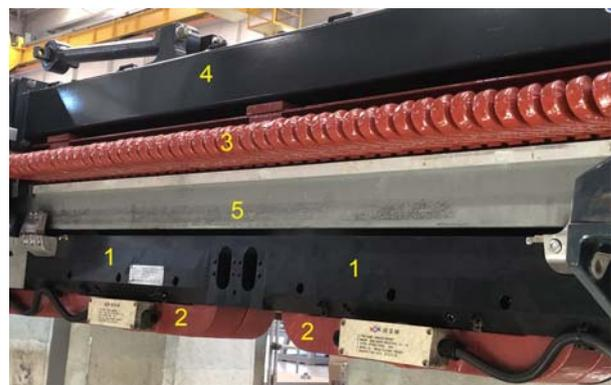
Fig. 7. Suspension electromagnets: 1 – steel core of the electromagnet, 2 – coil of the electromagnet, 3 – three-phase primary unit of the LIM, 4 – bogie of the car, 5 – steel reaction rail for suspension electromagnet (part 5 of Fig. 6). Photo taken in the maintenance depot.
