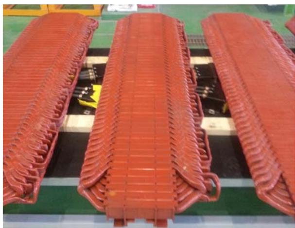
Fig. 9. LIMs for propulsion of IAML cars.
