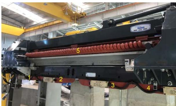
Fig. 8. Suspension-propulsion unit: 1,2,3,4 – electromagnets, 5 - three-phase winding of the primary unit of the LIM. Photo taken in the maintenance depot.
