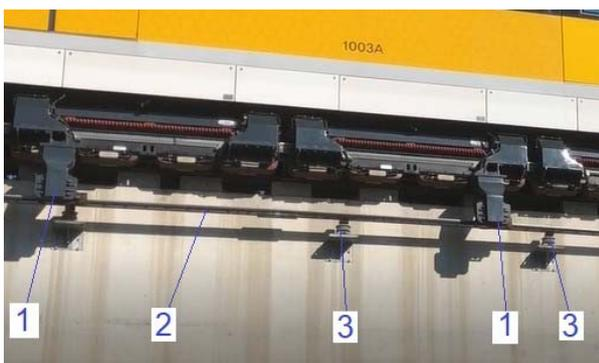
Fig. 5. Contact power transfer to vehicles: 1 – sliding contact mounted in the bogie, 2 – contact rail, 3 – insulator.
