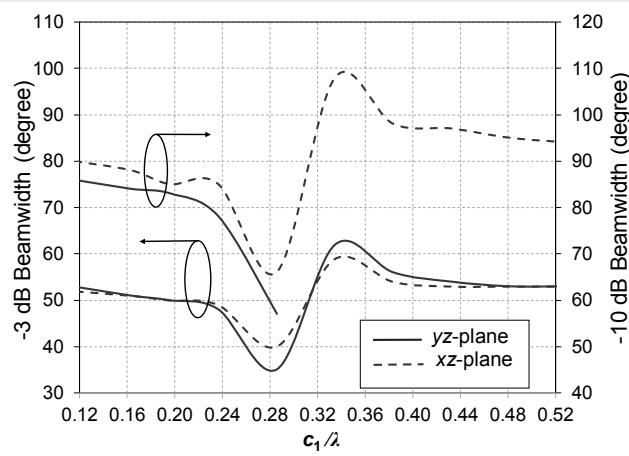
Fig.3. Simulated beamwidths of the OERW with FSCA for various lengths  $c_1$ .
