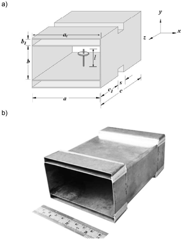
Fig.1. Geometry of the proposed antenna: (a) model and (b) prototype
