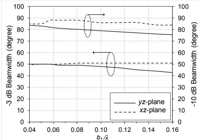
Fig.2. Simulated beamwidths of the OERW with FSCA for various height  $b_1$ .
