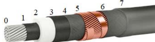
Fig.2. AXLPEP cable formation: 0 is the aluminium core; 1 is the core shield; 2 is the insulation; 3 is the insulation shield; 4 and 6 are cable paper; 5 is the copper shield; 7 is the cable sheath.
