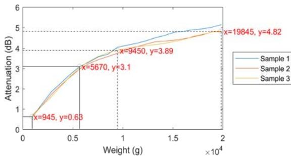
Fig.6. The damping characteristics of micro-bending sensors with 11 steel wires
