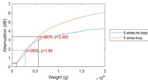
Fig.10. A comparison of the damping characteristics of micro-bending sensors with 5 steel wires – without a loop and with a loop
