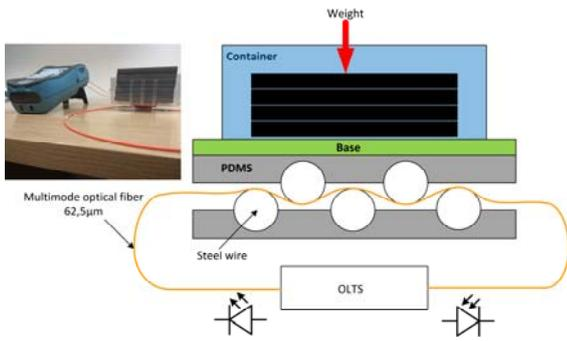
Fig.4. Layout of the measuring work space
