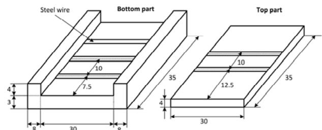
Fig.2. Dimensions of a micro-bending sensor with five steel wires
