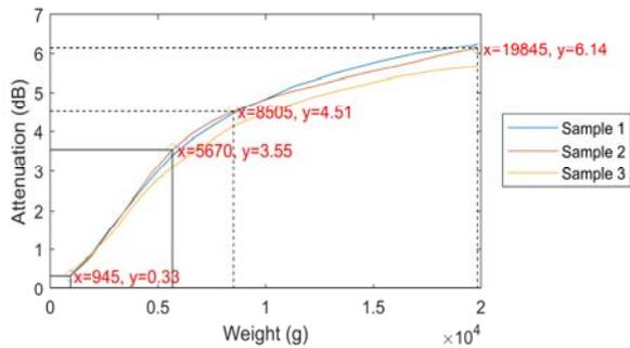
Fig.9. Damping characteristics of micro-bending sensors with 5 steel wires – layout of optic fibre in a loop
