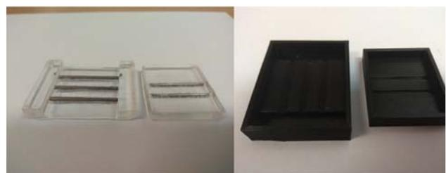
Fig.3. A micro-bending sensor made from PDMS and a casting form
