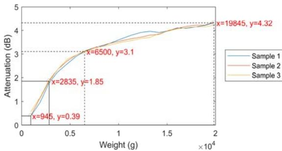
Fig.5. Damping characteristics of micro-bending sensors with 5 steel wires
