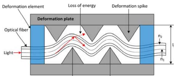
Fig.1. Typical layout of micro-bending sensor
