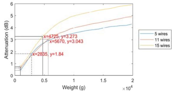
Fig.8. Comparing the damping characteristics of micro-bending sensors
