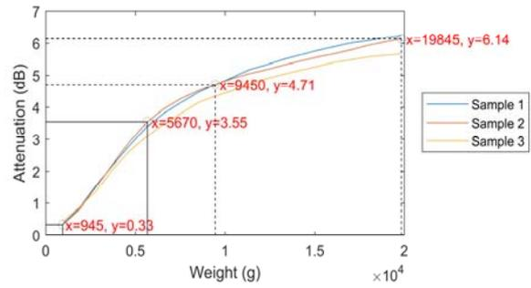
Fig.7. The damping characteristics of micro-bending sensors with 15 steel wires
