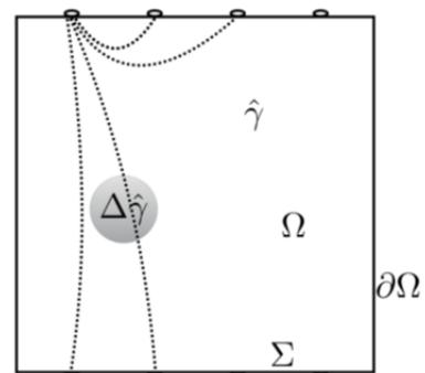
Fig. 3. Background domain with an object inside. The electrodes are placed at opposite boundaries,
