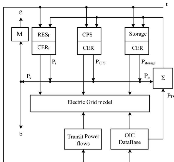
Fig. 4. Functional scheme of the most advantageous distribution of load between power plants
