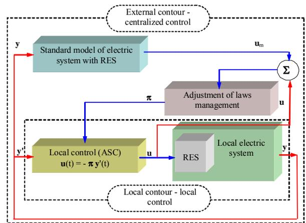
Fig. 2. Adaptive control system with the reference model
