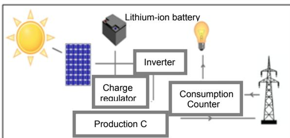
Fig.3. Solar energy conversion chain
