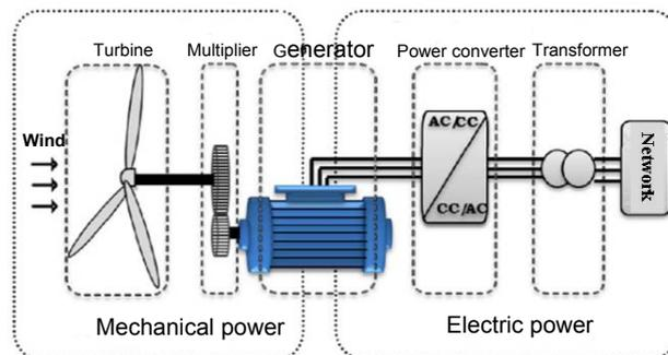
Fig.5. Principle of conversion of the kinetic energy of wind into electrical energy
