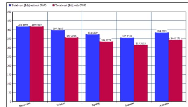
Fig.13. The charts of production capability and fuel costs of a combined Micro Gas Turbine and Solar systems without GWO, and with GWO.
