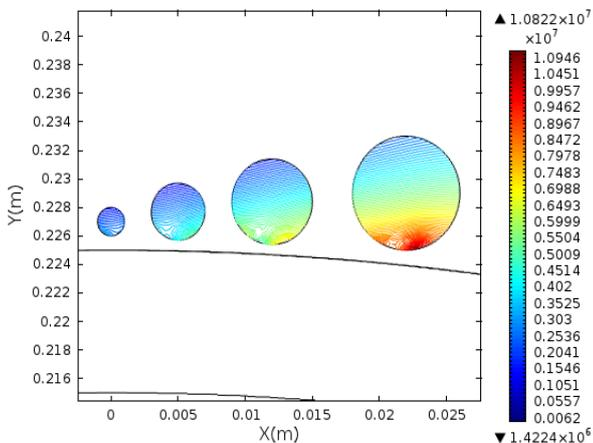
Fig. 4. Lorentz force orientation in conductive particle
