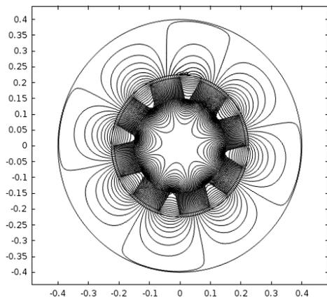
a- Magnetic vector potential A produced around (Wb/m)
