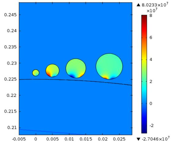
Fig. 5. Eddy current in Aluminum particles
