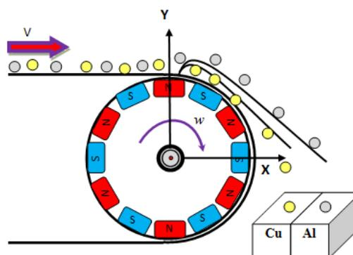
Fig. 1. Rotating eddy current separator
