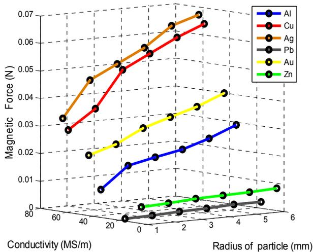
Fig. 6. Repulsive force of different kind of particles
