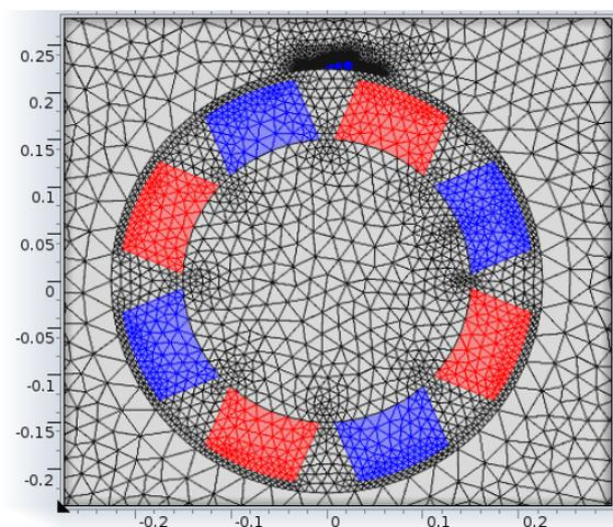
Fig. 2.. Meshing of separator with permanent magnets and particles.
