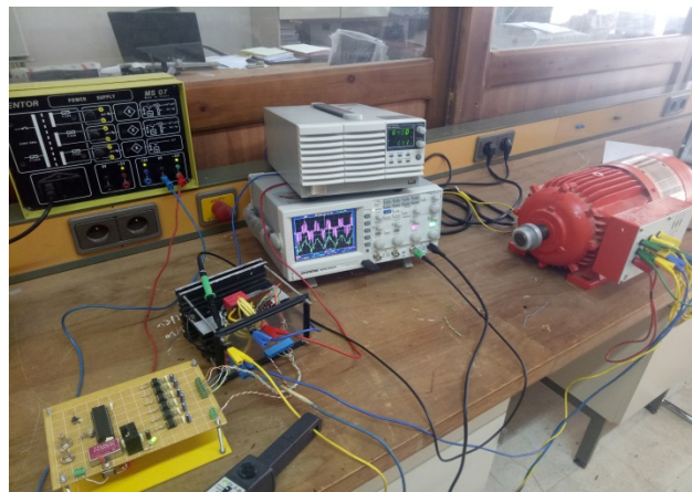
Fig.6. Hardware setup of three phase inverter fed to three phase induction motor
