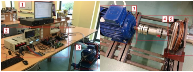
Fig.12. Developed test stand - photograph (1 - PC for programming and data processing; 2 - supply, DAQ and control system; 3 - six phase PMSM and encoder; 4 – torque measurement device; 5 - magnetorheological brake;)
