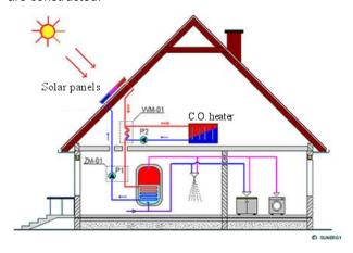
Fig. 5. The elements of heating system powered by via solar panels [8]
