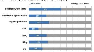
Fig. 3. The emission rates of toxic substances while burning blue coal as a percentage of emissions for regular black coal [5]
