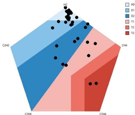
Fig. 6. Defects recognized by the Mansour pentagon method for data came from transformers in which partial discharges were found.
