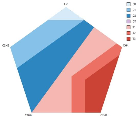
Fig. 4. Location of defect zones in the Mansour pentagon.
