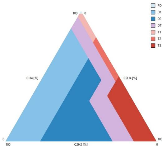
Fig. 2. Location of defect zones in the basic variant of the Duval triangle
