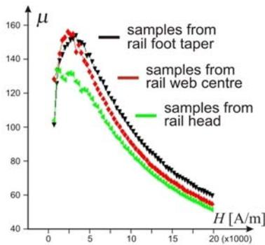
Fig.6 Relative magnetic permeability  $\mu = f_{\mu}(H)$
