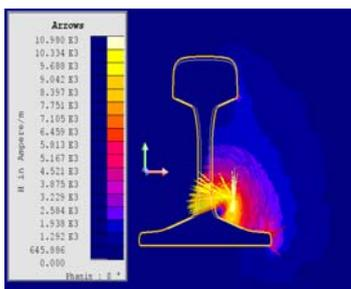
Fig.10. Graphic interpretation of the magnetic field intensity  $H$  distribution during rail induction heating in FEMM [11]
