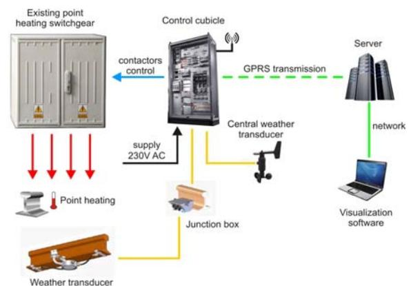
Fig.2 Electric resistance heating system of rail turnout
