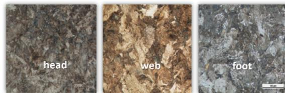
Fig. 5 Microstructure of rail steel [12]
