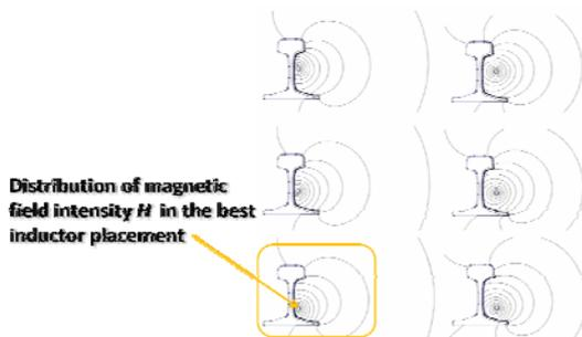
Fig.11. Influence of the inductor's placement on distribution of magnetic field intensity  $H$
