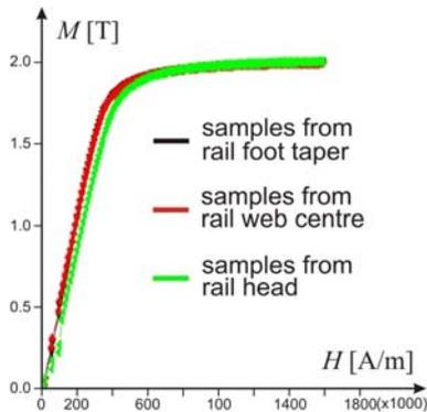
Fig.9. Magnetization curves  $M = f_M(H)$
