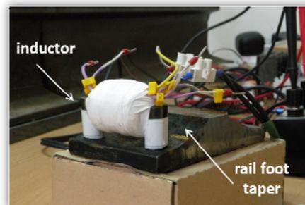
Fig. 12. The coil shaped inductor with a ferrite core (prototype)
