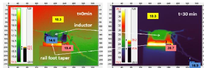
Fig.13. Thermal images of heated rail foot with the coil shaped inductor (number of coils  $z=150$ ,  $f=650\text{Hz}$ ,  $P=10\text{W}$ , 30 min of heating)
