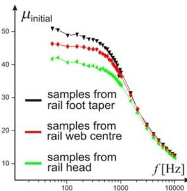
Fig.7. Initial relative magnetic permeability  $\mu_{initial} = f_{\mu_{initial}}(f)$
