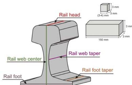
Fig.4 Locations of 60E1 rail testing samples
