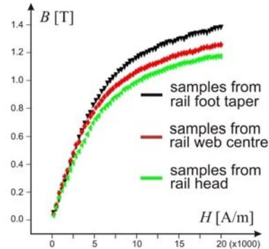
Fig.8 Prime magnetization curves  $B = f_B(H)$
