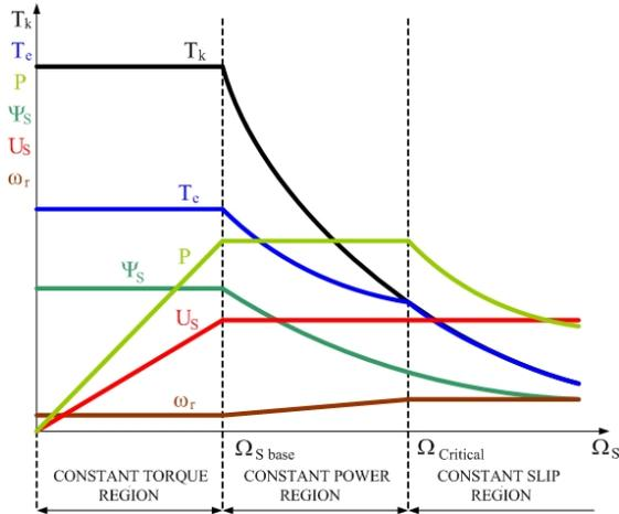
Fig. 16. Speed control ranges of AC traction drive: IM can operate in constant torque, constant power and constant slip regions whereas PMSM operates only in constant torque and constant power.
