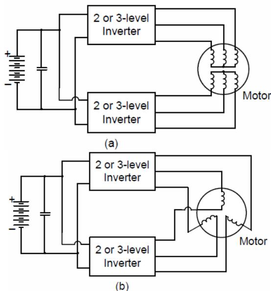
Fig. 12. Dual inverter topologies (a) parallel, (b) cascade
