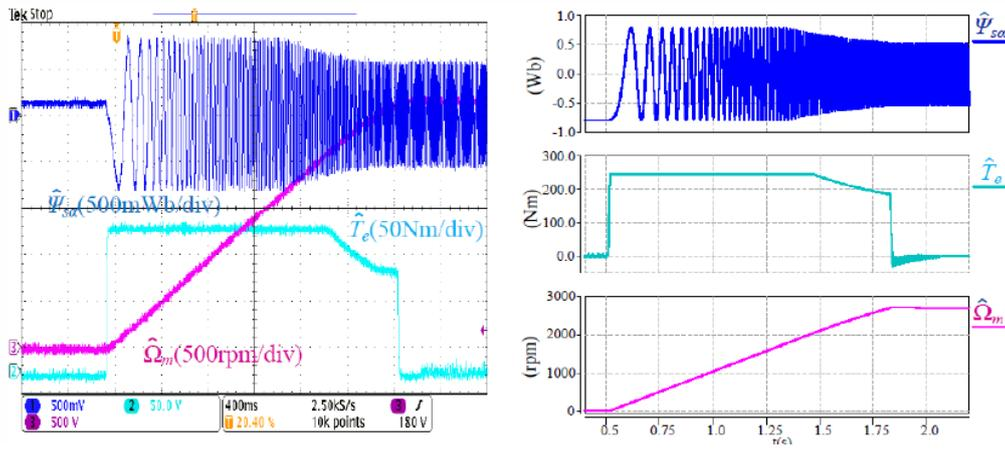
Fig. 19. Speed start-up till 2700obr/min in MPC controlled 50kW induction motor traction drive Left: experimental, right: simulation
