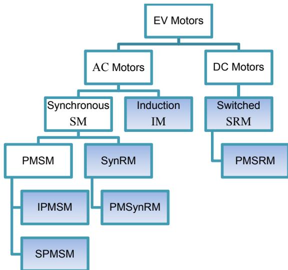
Fig. 2. Classification of motors used in electric vehicles. In the filled frames are motors discussed in this article.
