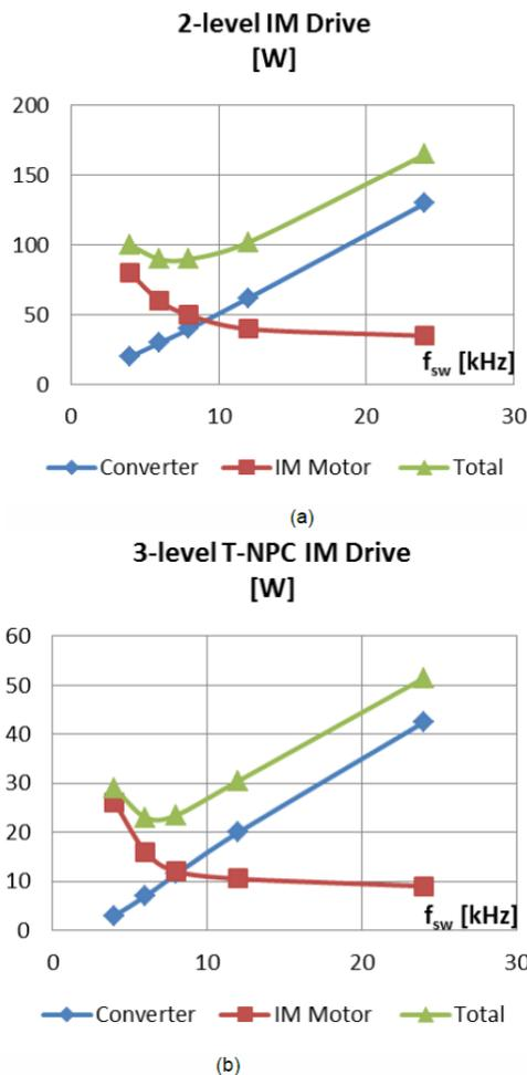
Fig. 14. Typical loss division between converter and IM motor in traction drives for two topologies: (a) 2-Level 6B, (b) 3-Level T-NPC
