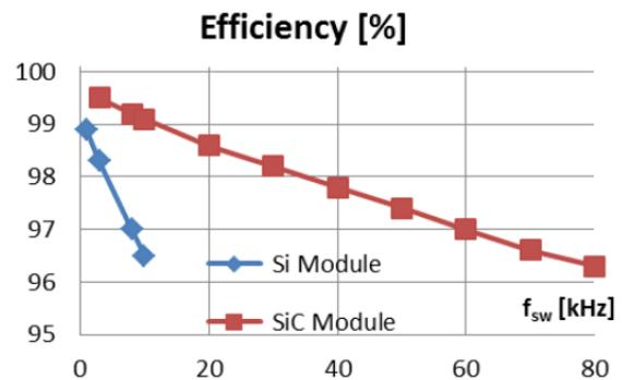
Fig. 9. Efficiency versus switching frequency of 100kW three-phase two-level converter with Si IGBT and SiC MOSFET power modules.
