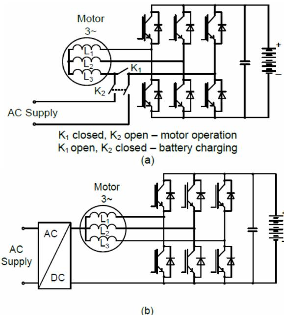
Fig. 13. Integrated motor-charger topology: a) with inverter used as AC active rectifier, b) inverter used as DC-DC converter
