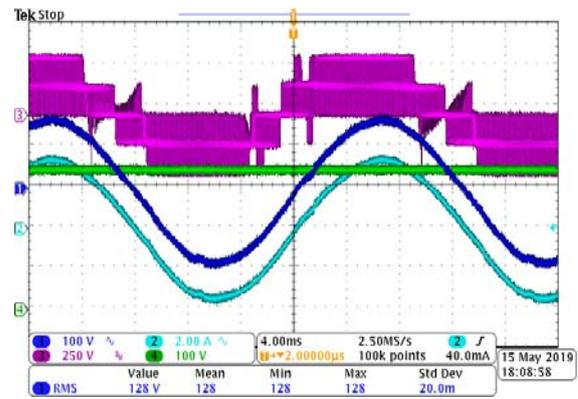
Fig. 11 (a) View of the 30kVA 3L-T-NPC prototype SiC converter, (b) typical waveforms under 40kHz switching frequency. From the top: line-line voltage, filtered voltage, output current, DC link voltage.
