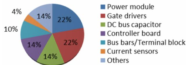
Fig. 8. Typical percentage division of the traction inverter costs for BEV [37]
