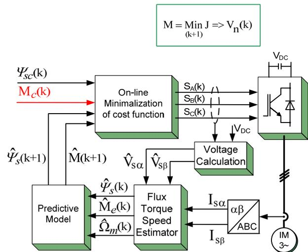
Fig. 18. Block scheme of model predictive torque and flux control (MPC-PTC)
