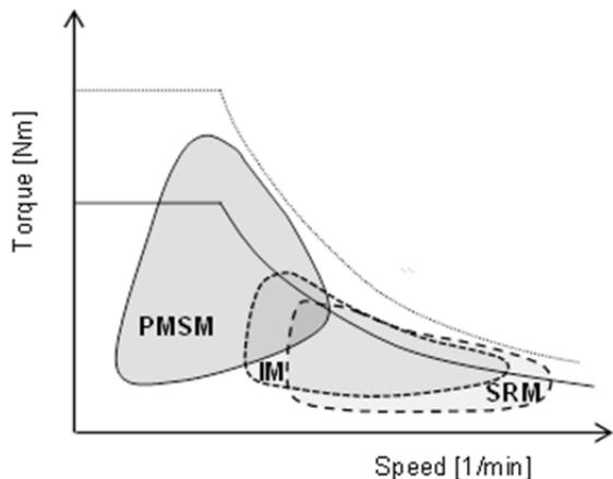
Fig. 6. Efficiency maps of different machines. The areas of every kind of motor have the efficiency >85%
