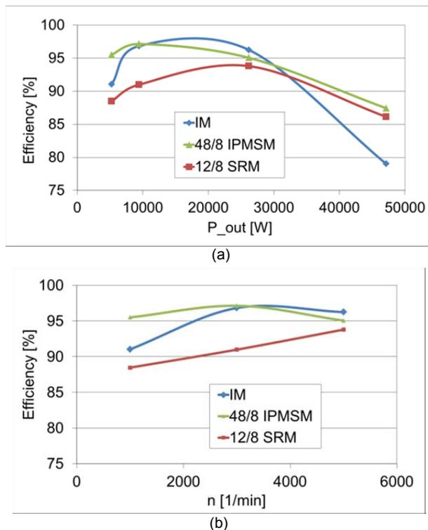
Fig. 7. Characteristics of efficiency for different motor types versus (a) output power  $P_{out}$  and (b) speed
