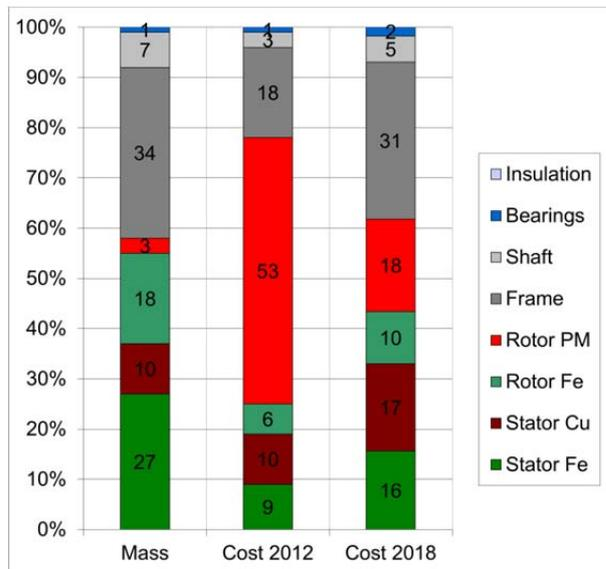
Fig. 5. Percentage of PM motor components (rated power 80 kW) in total weight and their share in the total cost in 2012 year, when the price of rare-earth magnets was the highest 500 \$/kg and in 2018 year, when the price of rare-earth magnets was 100 \$/kg
