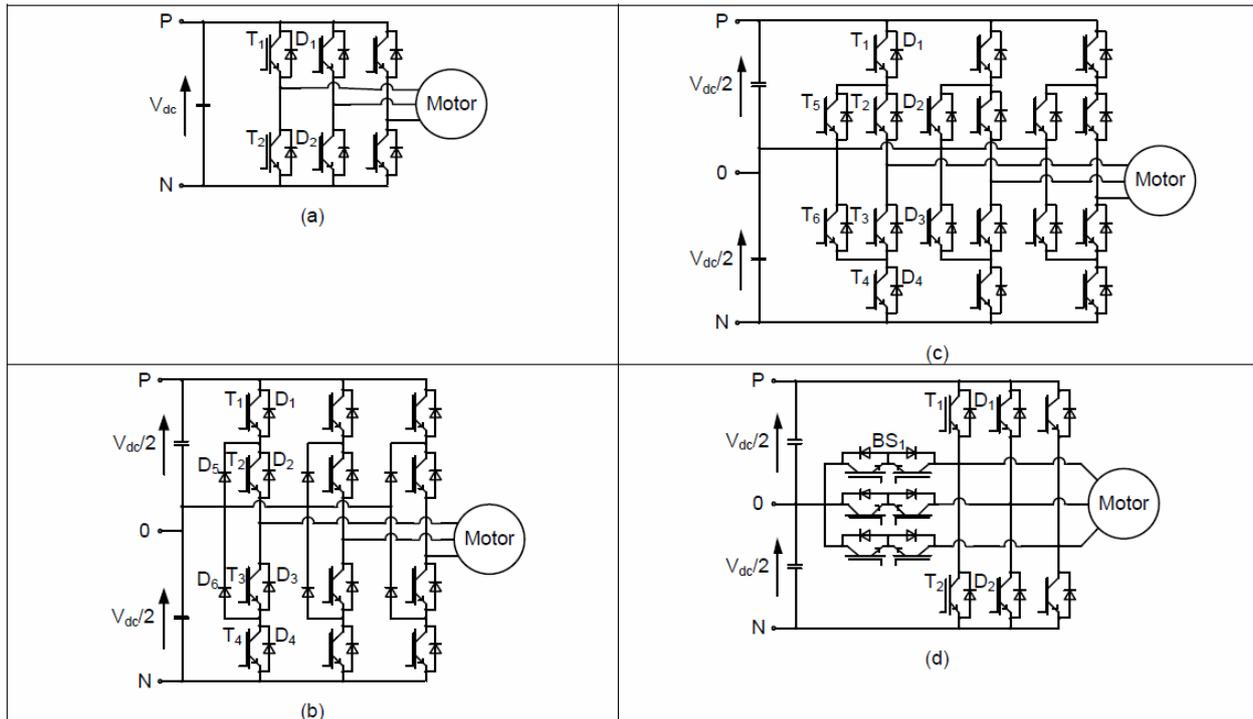
Fig. 10. Basic topologies of traction converters for electric cars, (a) 2-Level bridge 2L, (b) 3-Level Diode Neutral Clamped Converter D-NPC, (c) 3-Level Active Neutral Point Clamped Converter A-NPC (d) 3-level Transistor Neutral Point Clamped Converter T-NPC (also known as T-Type Converter).
