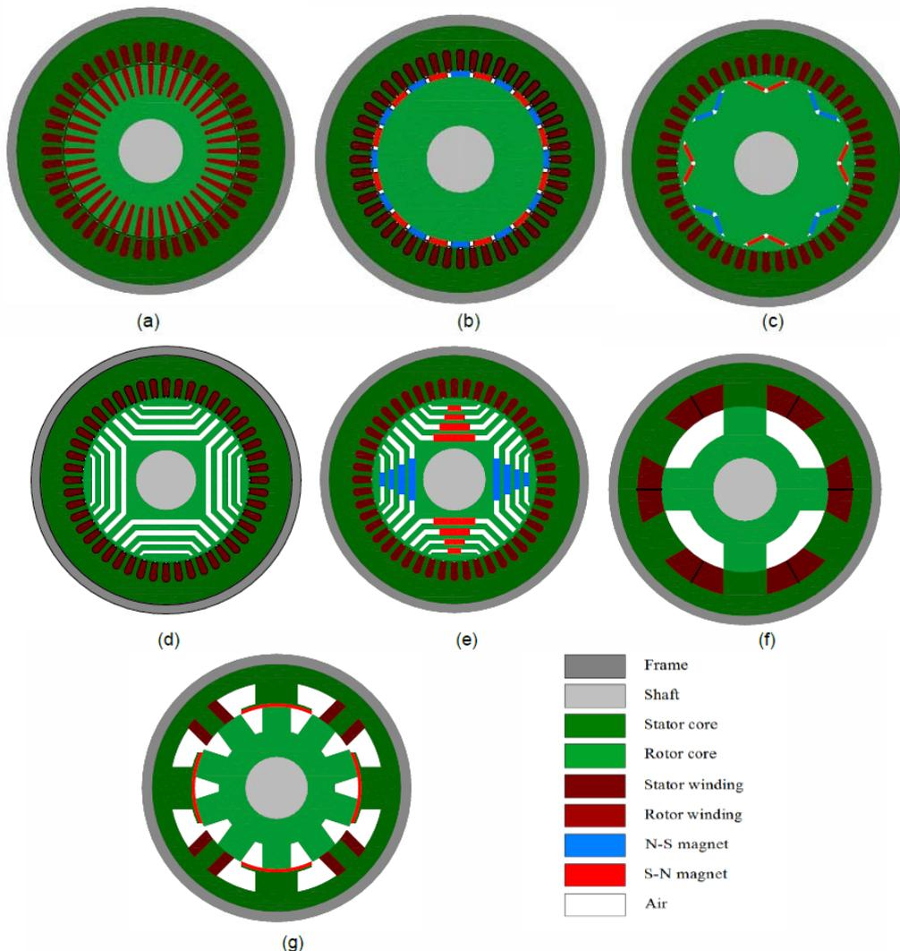
Fig. 3. Types of motors used in electric vehicle drives: (a) squirrel-cage induction motor (IM), (b) surface PMSM, (c) internal PMSM, (d) Synchronous reluctance motors (SynRM), (e) Synchronous reluctance motors with permanent magnets (PMSynRM), (f) Switched reluctance motors (SRM), (g) Switched reluctance motors with permanent magnets (PMSRM)
