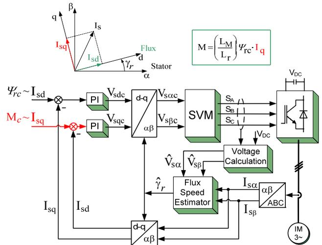
Fig. 17. Block scheme and vector diagram of torque and flux control in the Field Oriented Control (FOC) method.
