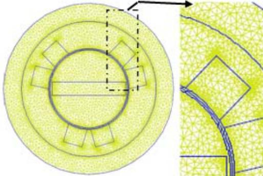
Fig 4. 2D FEM mesh for the HTS RM
