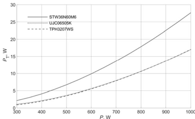
Fig. 11. Calculated total power loss in a single transistor as a function of output power of the converter at a switching frequency of 500 kHz and junction temperature of 25°C
