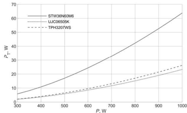
Fig. 10. Calculated total power loss in a single transistor as a function of output power of the converter at a switching frequency of 300 kHz and junction temperature of 150°C
