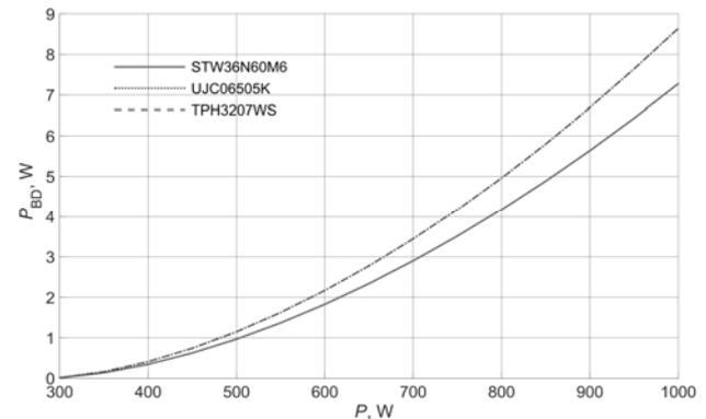
Fig. 8. Calculated freewheeling diode conduction loss in a single transistor as a function of output power of the converter at a switching frequency of 500 kHz
