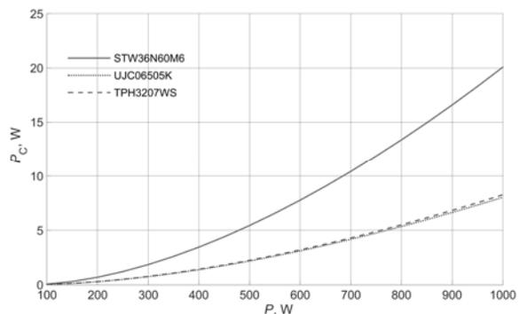
Fig. 3. Calculated conduction loss in a single transistor as a function of output power of the converter at a switching frequency of 500 kHz and junction temperature of 25
