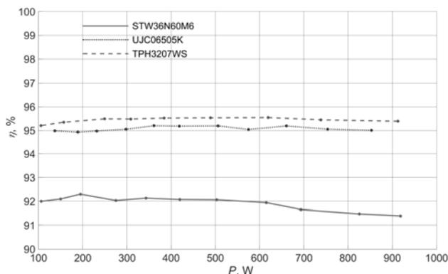
Fig. 16. Overall efficiency of the converter for each of the examined FETs as a function of output power at a switching frequency of 400 kHz
