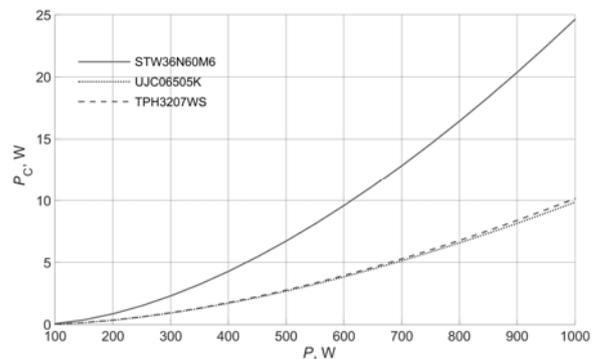
Fig. 2. Calculated conduction loss in a single transistor as a function of output power of the converter at a switching frequency of 300 kHz and junction temperature of 25°C
