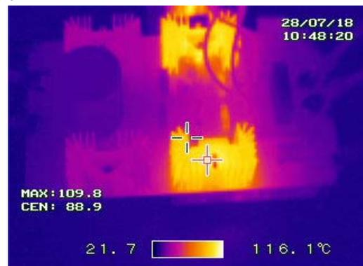
Fig. 13. Infrared photograph of the converter with STW36N60M6 silicon transistors at the nominal output power
