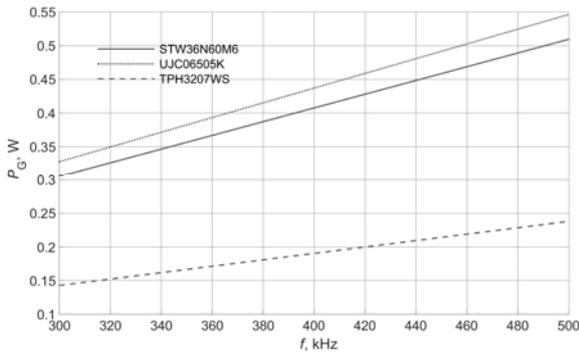
Fig. 6. Calculated gate loss in a single transistor as a function of switching frequency
