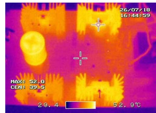
Fig. 14. Infrared photograph of the converter with UJC06505K silicon carbide transistors at the nominal output power
