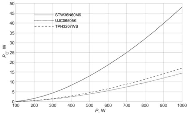
Fig. 5. Calculated conduction loss in a single transistor as a function of output power of the converter at a switching frequency of 500 kHz and junction temperature of 150°C
