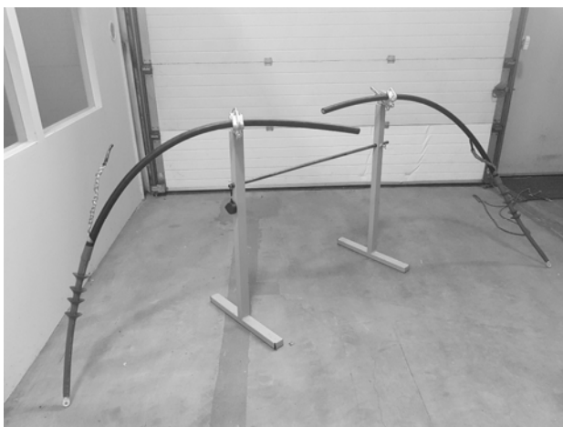
Fig.2. Preparation of the test specimens: cable before an assembly of the tested joints and after PD measurements
