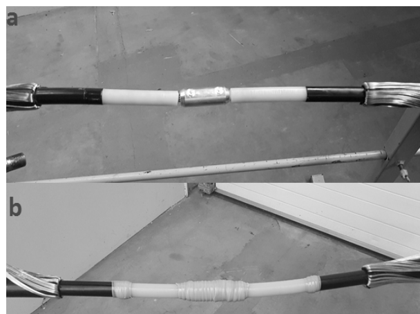
Fig.3. Preparation of the test specimens: a) connector before and b) after assembly of stress control mastic for test specimen No. 1
