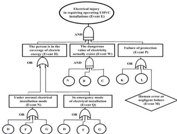
Fig. 1 – Model of the "event tree" of electrical trauma development during hot work in UHVC electrical installations.
