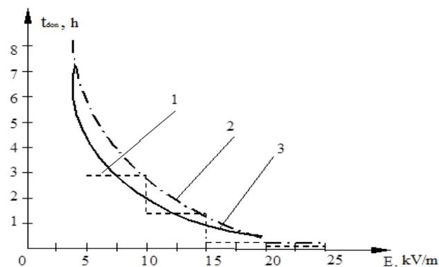
Fig. 3 – Graphs of dependences of the allowable time of stay in an electric field on the intensity of IFEF
