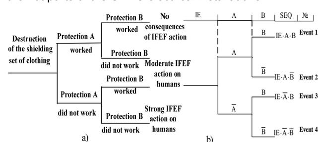
Fig. 2 – "Failure tree" model for the case of shielding clothing damage when working on UHVC airline wires (a) and a formal representation of the "failure tree" for the specified case (b)
