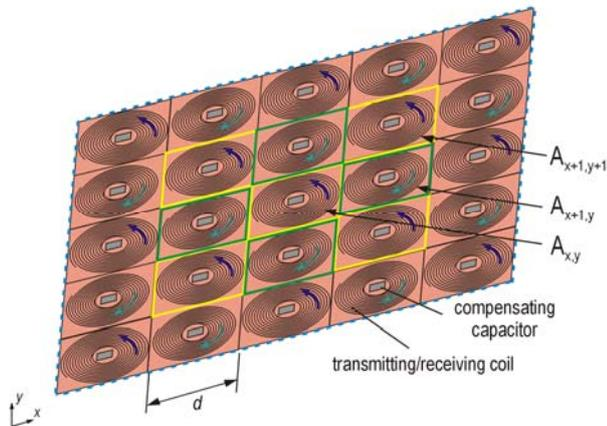
Fig.2. A two-dimensional network transmitting/receiving surface of the non-periodic WPT system ( $A_{x,y}$  – the WPT cell)
