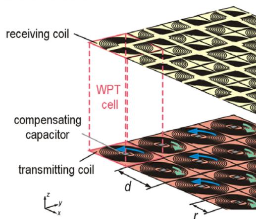
Fig.1. A view on an analysed WPT system
