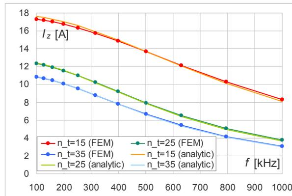
Fig.5. Results comparison of source current ( $I_z$ ) dependent of number of turns ( $n_t$ ) for the case  $h = 10 \text{ mm}$
