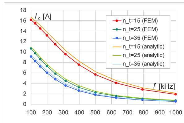
Fig.4. Results comparison of source current ( $I_z$ ) dependent of number of turns ( $n_t$ ) for the case  $h = 5 \text{ mm}$
