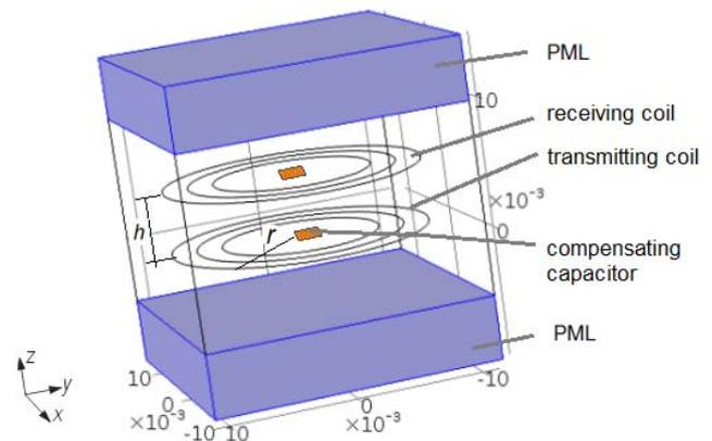
Fig.3. A three-dimensional view on one of WPT cell
