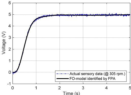
Fig.5. Results of fractional-order model identification of BLDC motor [28]
