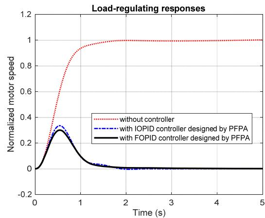
Fig.9. Unit-step load-regulating responses of the BLDC motor speed control system without and with IOPID and FOPIID controllers designed by PFPA
