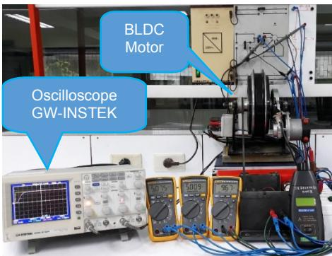
Fig.4. BLDC motor testing rig
