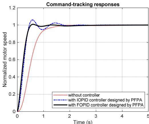
Fig.8. Unit-step command-tracking responses of the BLDC motor speed control system without and with IOPID and FOPIID controllers designed by PFPA
