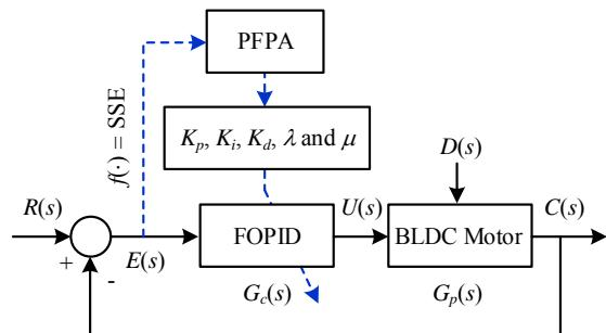
Fig.7. FOPIID design framework for BLDC motor speed control by PFPA
