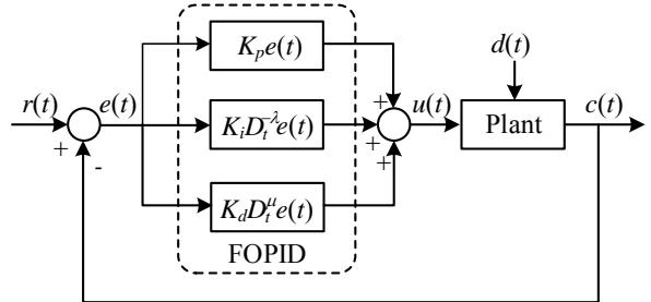
Fig.6. FOPIID feedback control loop
