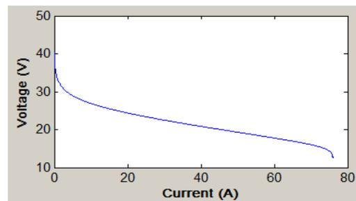
Fig.3. Polarisation curve of a Ballard Mark V PEM Fuel cell stack
