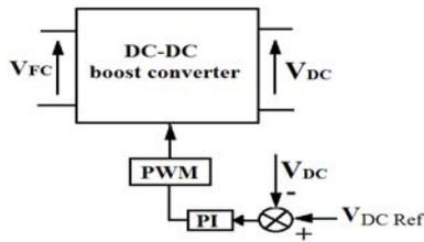
Fig.4. DC/DC converter control
