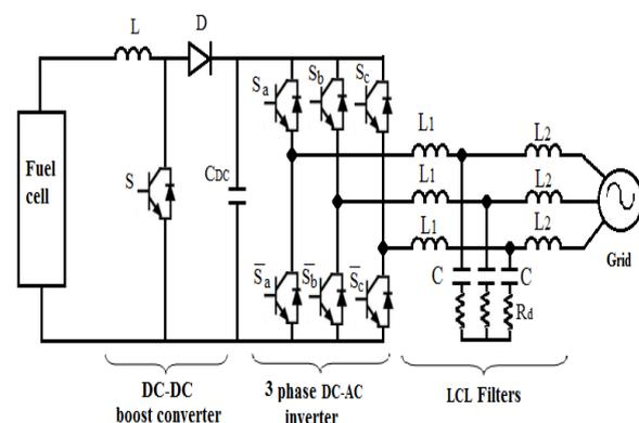
Fig.1. Proposed fuel cell grid connected system
