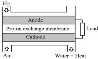
Fig.2. PEM fuel cell principle
