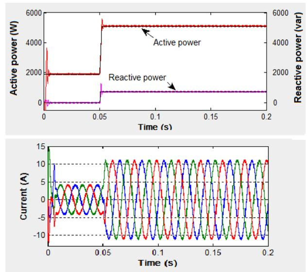
Fig.7. Active/reactive power and grid injected current
