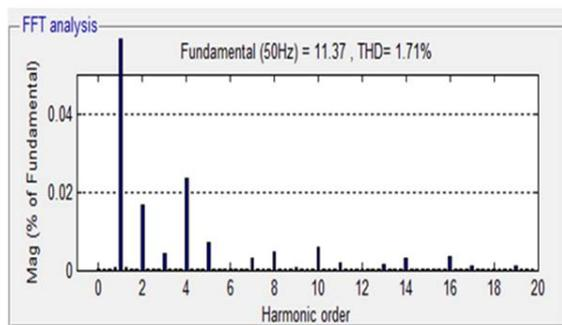
Fig.8. Injected current harmonic spectrum
