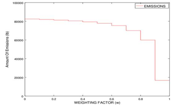
Fig. 3. Impact of Varying Weighting Factor on Emissions
