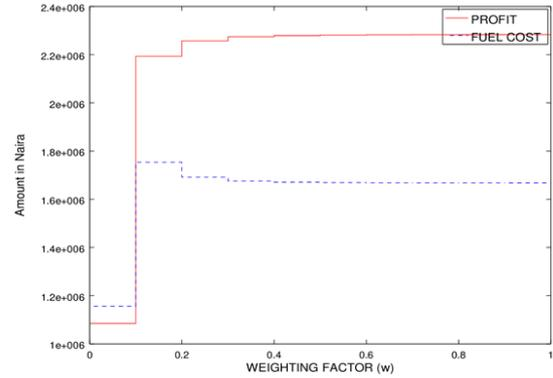
Fig. 2. Impact of Varying Weighting Factor on Profit and Fuel Cost
