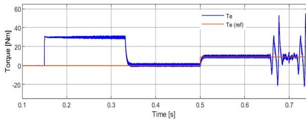
Fig.2. Torque response of induction motor controlled with DTC-SVM under healthy and faulty condition of MC.
