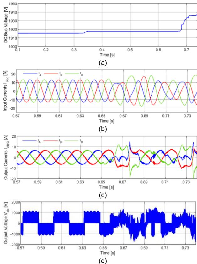
Fig.3. Currents and voltages in MC under healthy and faulty conditions (a) DC bus voltage of Clamp Circuit, (b) three-phase input currents, (c) three-phase output currents, and (d) line-to-line output voltages.
