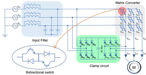
Fig.1. Induction machine drive-based matrix frequency converter
