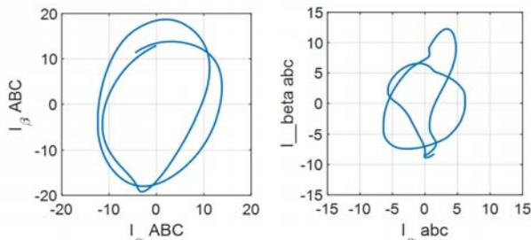
Fig.5. Input and output currents in Concordia frame with a faulty switch.
