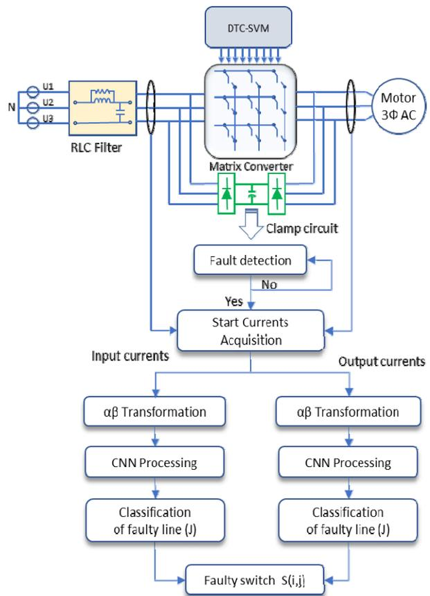
Fig.4. Proposed detection and localization method structure of a matrix frequency converter
