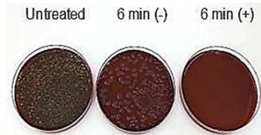
Fig. 19. Photography comparing negative and positive polarity treatment effect. Corona Voltage = 25 kV, Interelectrodes distance = 30 mm
