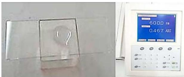
Fig. 3. Photography of *E. coli* liquid drop with optical density in the spectrometer UV-mini 1240.
