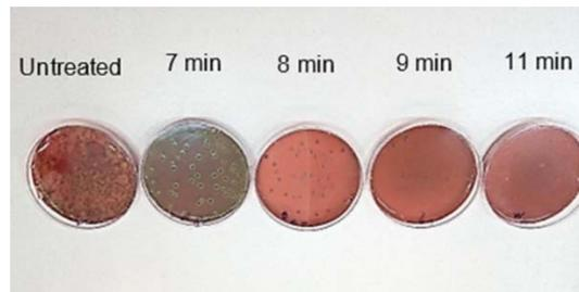
Fig. 5. Photography of bacterial load as a function of plasma treatment time
