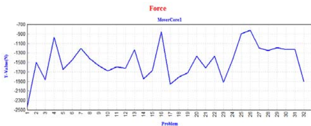
Fig. 8 Dependence of the constituent of the force on the movable part on the axis Oy from the position of the movable part with respect to the permanent magnets at an inclination angle \alpha=30^\circ .
