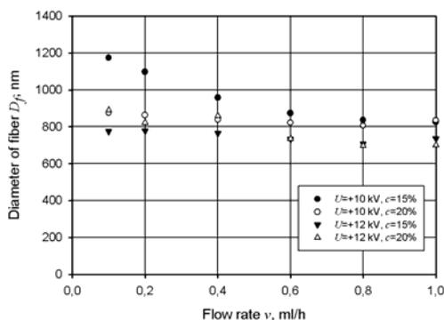
Fig.6. Influence of the flow rate of polymer solution on the diameter of fibers for different conditions of the process. Results obtained for capillary diameter  $d=0.5$  mm, distance between the capillary and collector  $l=120$  mm in the air
