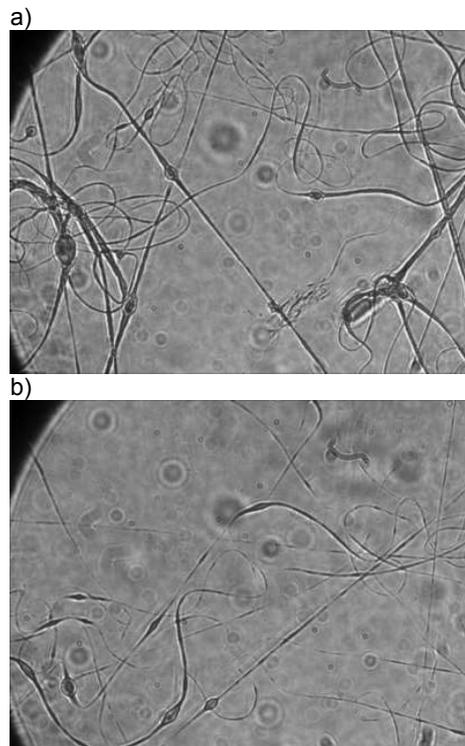
Fig.5. Optical image of PVDF fibers with beaded morphology. Results obtained for capillary diameter  $d=0.5$  mm, applied voltage  $U=+14$  kV, distance between the capillary and collector  $l=120$  mm, and flow rate  $v=1$  ml/h in the air: a) PVDF concentration  $c=20\%$ , b) PVDF concentration  $c=15\%$
