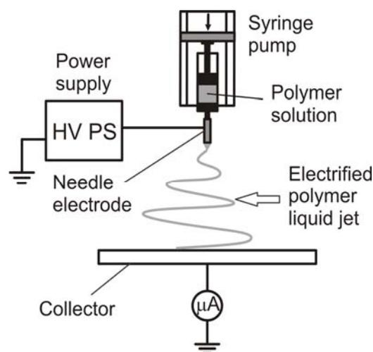
Fig.1. Scheme of the experimental system for the fabrication of polymeric nanofibers and measurement of current-voltage characteristics of electrospinning process
