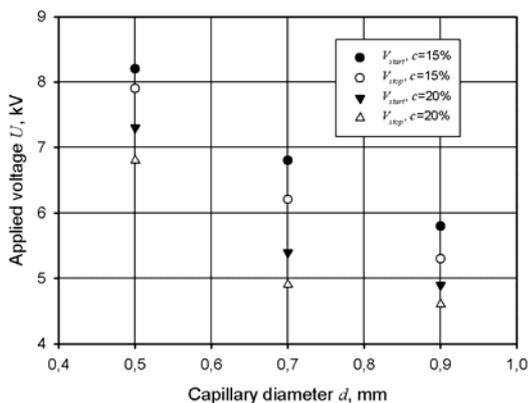
Fig.7. Influence of capillary diameter  $d$  on the behaviour of electrospinning process. Results obtained for applied voltage  $U=+12$  kV, distance between the capillary and collector  $l=120$  mm, and flow rate  $v=1$  ml/h in the air
