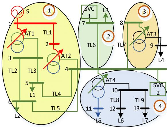
Fig.3. EPS test circuit, AT – autotransformer, TL – transmission line, L – load, SVC – Static Var Compensation, S – external system
