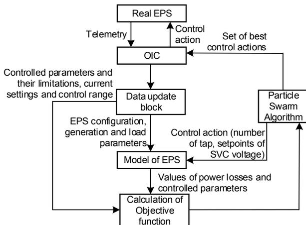
Fig.2. Block diagram of the proposed voltage and reactive power control system
