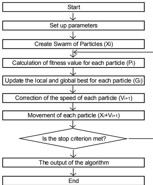
Fig.1. Flowchart of Particle Swarm Optimization
