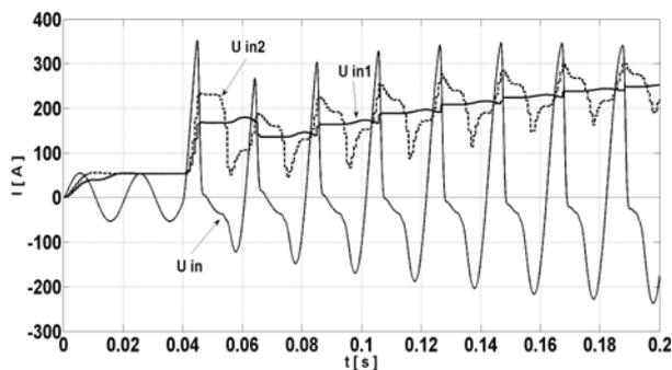
Fig.7 The effect of the DF with window of observation is equal to half of the period of fundamental frequency
