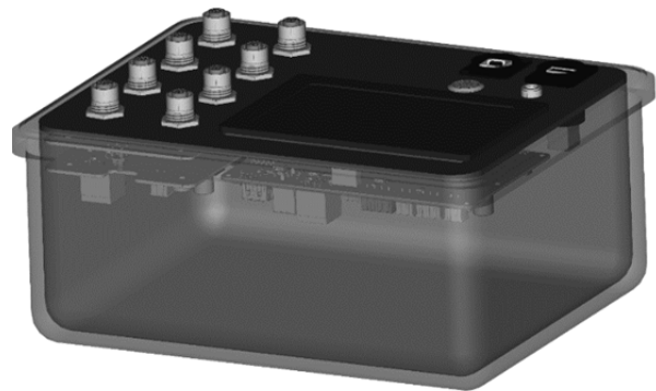
Fig. 5. Tomograph mounting concept in a peile case - side view.
