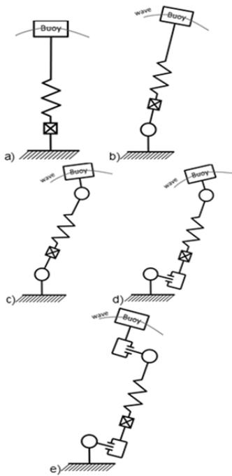
Fig.2. 1-DoF (a), 2-DoF (b), 3-DoF (c), 4-DoF (d), 5-DoF (e)
