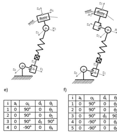
Fig.3. 1-DoF (a), 2-DoF (b), 3-DoF (c,d), 4-DoF (e), 5-DoF (f) kinematic chain of the buoy movement with kinematic parameters tables
