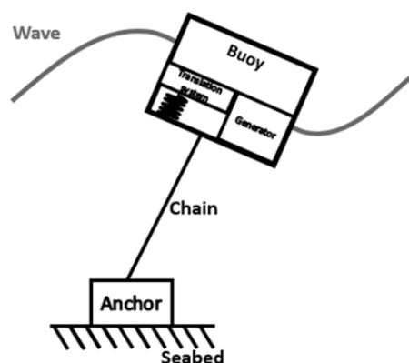
Fig.1. The Power Buoy model
