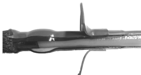
Fig. 2. Part of sectioned modeled termination with visible semiconducting mastic (yellow) and semiconducting tube (black).
