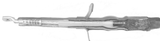
Fig. 1. General view of examined cable termination
