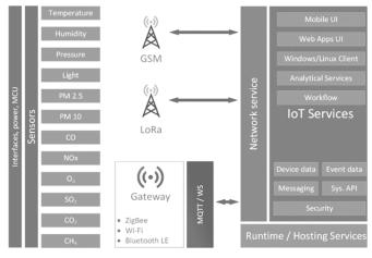
Fig. 1. Schema of sensors IoT operational blocks.
